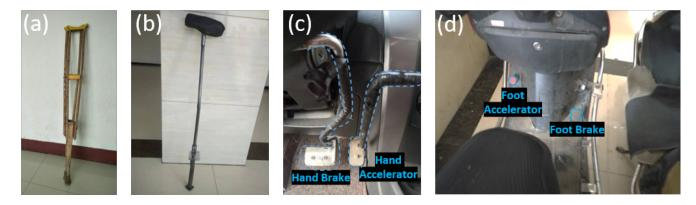
Figure 2: (a,b) Self-made crutches which lack careful design and engineering considerations. (c) Accessibility modifications made to a car by a third-party company for a participant with motor impairment. (d) Self-modified brake and accelerator of the motorcycle of P6 (no forearm).
